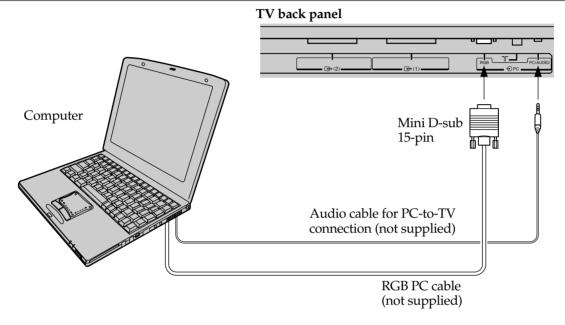
Connect a PC cable from the computer to the RGB/PC input terminal on the back of the TV.
